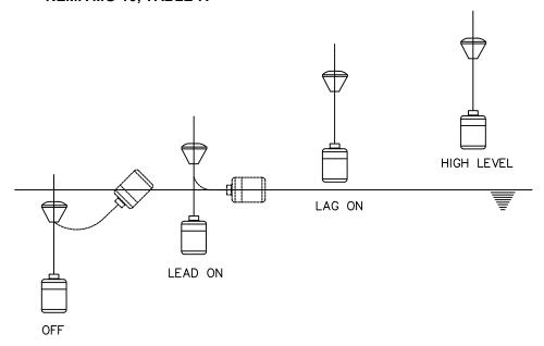
Figure 4: Float Switch Installation
