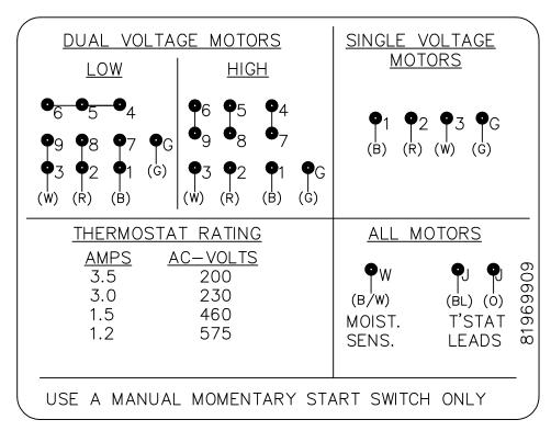
Figure 5: Motor Connection Diagram
