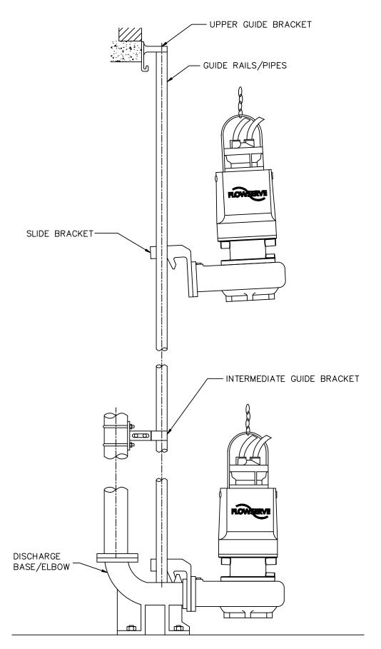
Figure 1: Guide Rail System
