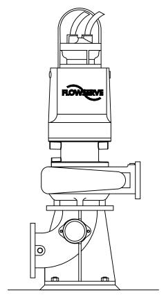
Figure 2: Dry Pit Installation
