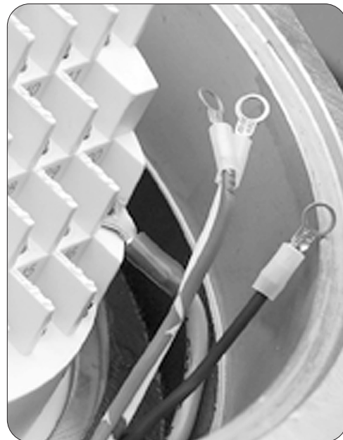
Figure 3.15: Ring tongue connectors
