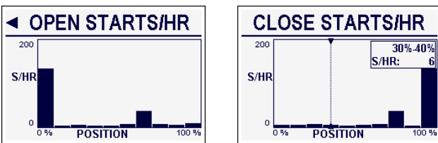
Figure 7.10: Open and close starts/hr histograms. Close starts/hr histogram displays optional bin s/hr and position values.
