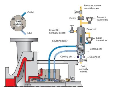
Plan 54: Dual seal circulation from an external source
