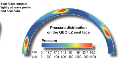
Pressure generated at the wave peaks can be several times higher than the seal chamber pressure, suppressing vaporization and maintaining stablity in the area of contact.
