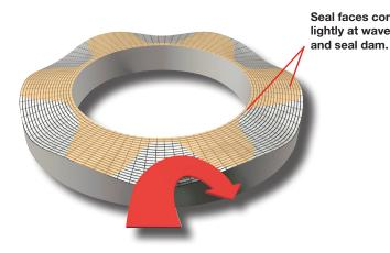
Process fluid enters the wave valley, fluid is pressurized at the wave peaks, vapor is driven back into a liquid state, and fluid recirculates back into the seal chamber.
