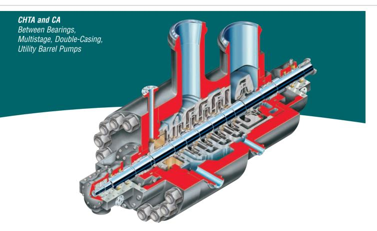
The advanced design of the CHTA and CA high-pressure barrel pumps has been developed and refined through more than 50 years of experience. Flowserve uses industry-leading technology throughout every aspect of design and manufacturing to produce the most reliable high-energy boiler feed pumps in the world. The design of the model CHTA and CA incorporates hydraulic and mechanical features resulting from many years of experience in building this class of equipment.
