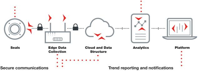
The system architecture collects data from equipment sensors and transmits it via a secure encrypted network.
