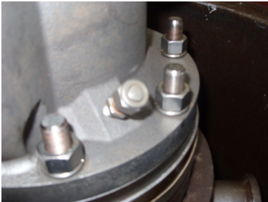
Fig. 5.2.9b Oil Line connection port to the motor
