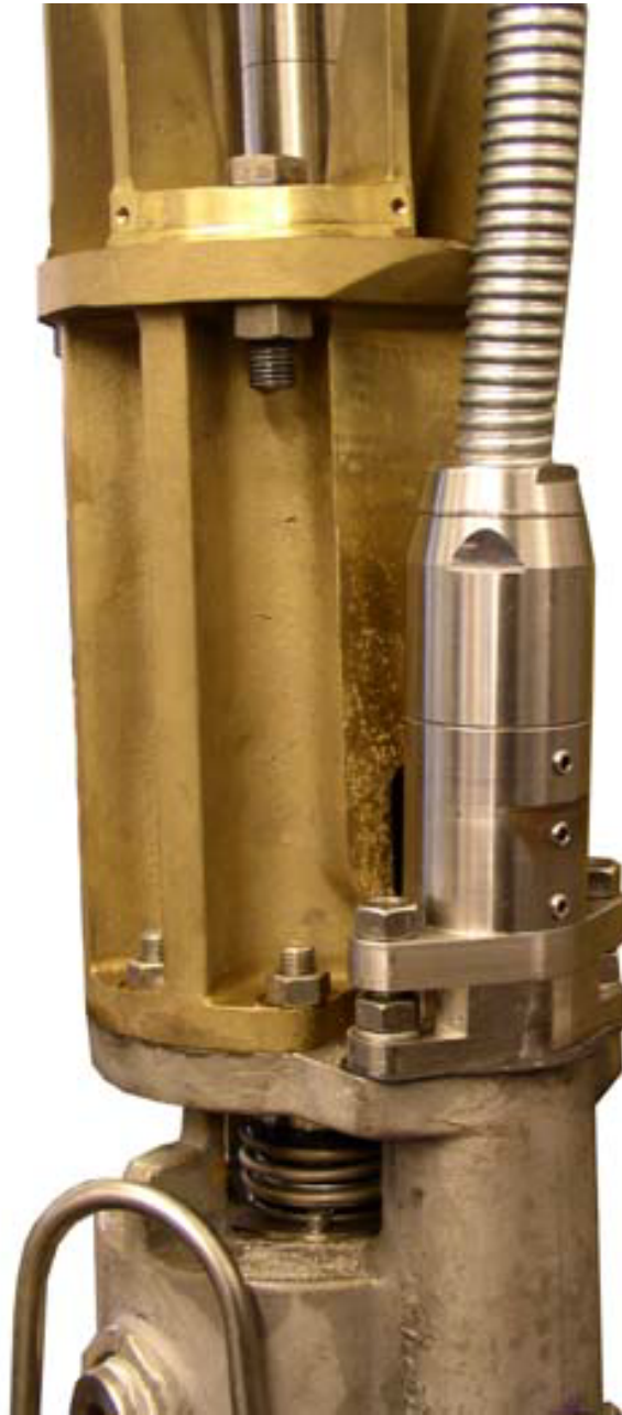
Figure 5.2.8c Variant B- Metal Housing Motor Lead Extension with Flanged Connection
