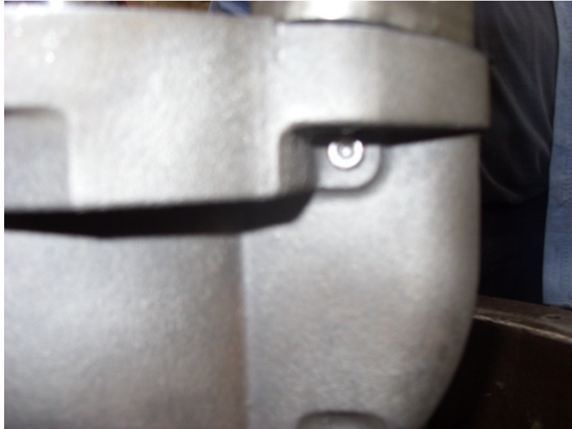
Fig. 5.2.9.c Motor Vent Screw Location in Top Case
