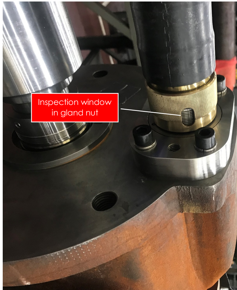
Fig. 5.2.8.m Inspection window with fully tightened MLE gland nut
