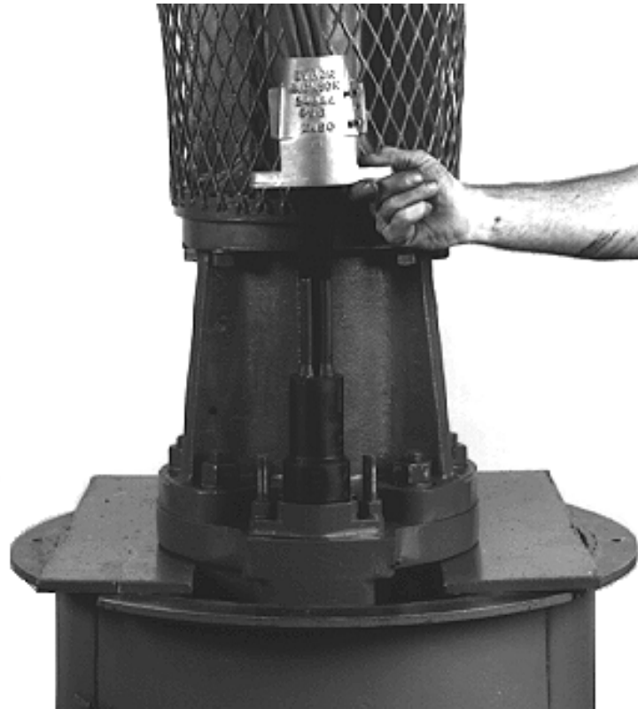
Figure 5.2.8g Molded Plug installed and slide clamp to fit over molded plug
