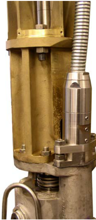
Figure 5.2.8i Metal housing power terminal connector with bolted connection (3300 V-cable or higher)
