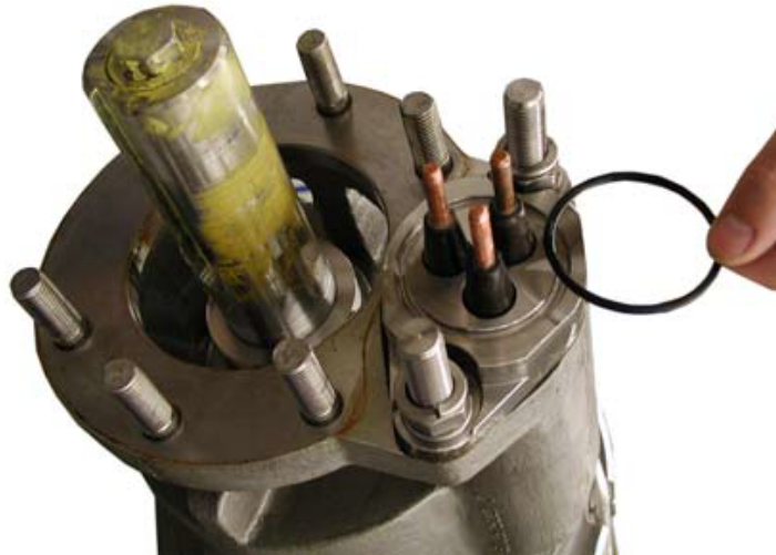
Figure 5.2.8.j O-ring for metal housing power terminal connector at motor gland plate (3300 V or higher)
