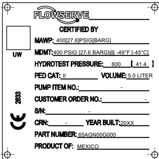
Figure 2: Example of typical nameplate
