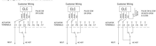
All wiring to terminal strip should be inserted only to midpoint of terminal strip.
