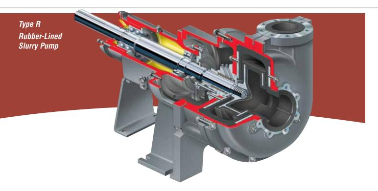
The type R rubber-lined slurry pump is a horizontal, single-stage, end suction design, with a tangential discharge nozzle. Engineered to handle high concentrations of fine abrasive solids in suspension or corrosive and abrasive mixtures, the R pump is a workhorse in solids handling industries.
