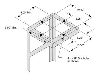
1.5 Carefully place the Airfin Cooler on the mounting bracket. The Airfin Cooler should be positioned so that the least amount of elbows or tube bends are needed for the inlet and outlet piping.
