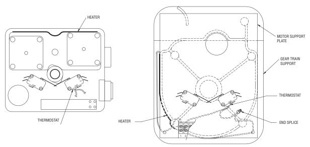
Figure 3—Wiring for 10-30 H75 Heater/Thermostat Option
