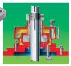
This bearing configuration allows use of standard motors for high horsepower or ultra-high thrust operating conditions. The bearings are lubricated by oil and controlled by a lube oil system.
