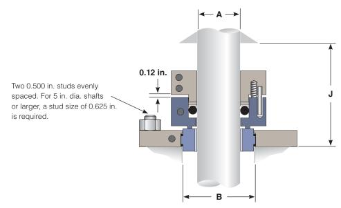
**Note:** Dimension J reflects the minimum distance required for the assembled seal plus additional axial space required for seal assembly.
