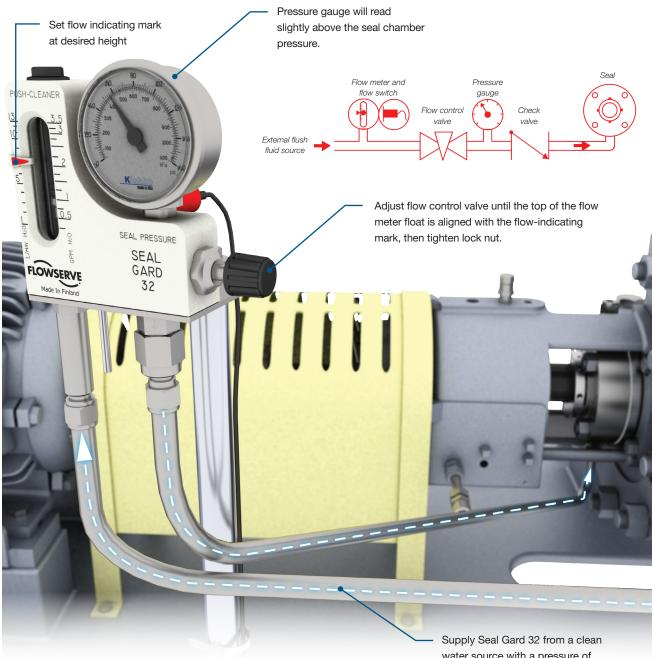
Supply Seal Gard 32 from a clear water source with a pressure of 1 bar (14.5 psi) higher than the seal chamber pressure.
