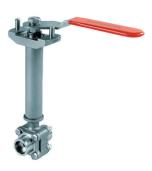
Provide reliable shutoff in intermittant or continuous cyrogenic applications down to -254°C (-425°F) with this three-piece, flanged ball valve specifically designed for liquefied gases.
