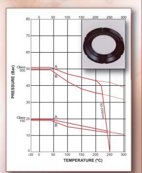
**Key** *A* = Carbon Steel Body Rating *B* = Stainless Steel Body Rating (In accordance with BS1560 / EN 1759)
