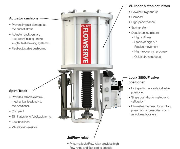
JetFlow relay delivers proportional pneumatic output for both precision control for small step changes, and high flow when fast speeds
