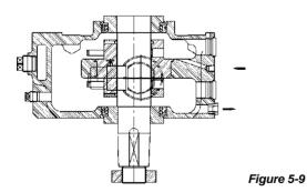
Remove inlet and outlet pipe plugs from the above connections. Install appropriate re-classifier in the top opening, leave open vent connections, connect oil recovery trap to bottom opening or leave it open to act as a relief. Refer to figure 5.8 and 5.9 for details.
