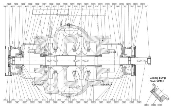
8.5.1 HED-DS with anti-friction bearing, oil mist lubrication and fan cooling parts list
