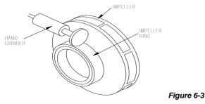
b) Make sure ring fits on impeller are free of nicks or burrs. Heat new ring to 107 °C (225 °F) and install on impeller. Drill and tap new holes in impeller spaced half the circular distance from the previously used holes in the impeller. (See figure 6-4.)
