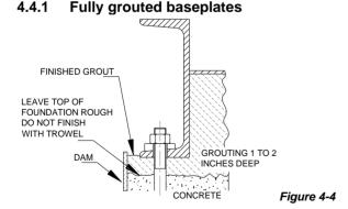
Use a good, high strength, non-shrink grout mix and install as in the manufacturer's instructions.
