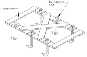
Figure 4-1: template for hanging foundation bolts
