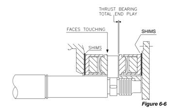
m) Fit O-ring in place, install thrust bearing outer cover and tighten bolting.
