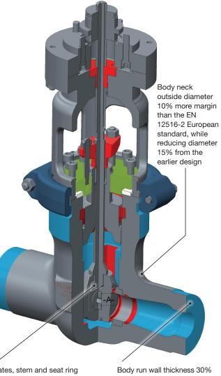
Gates, stem and seat ring designed to withstand requirements of higher allowable pressures of EN 12516-2 Body run wall thickness 30% more margin than EN 12516-2, while reducing diameter 50% from the earlier design
