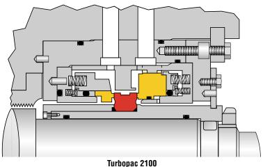
double mechanical seal in a face to face arrangement for high pressure applications
