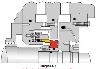
single mechanical seal with reverse pressure capability and floating ring seal on the atmospheric side
