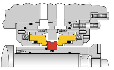
Turbopac 368 double mechanical seal in a face to face arrangement
