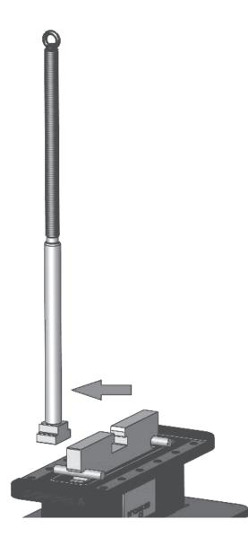
Figure 12 - Stem head disengaging.
