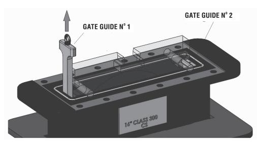
Figure 13 - Gate guides removal
