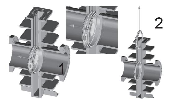
Figure 17 - Seat disassembly from the body
