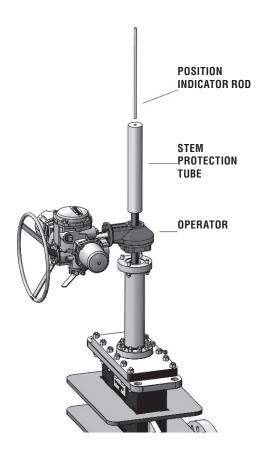
Figure 7 Operator removal sequence
