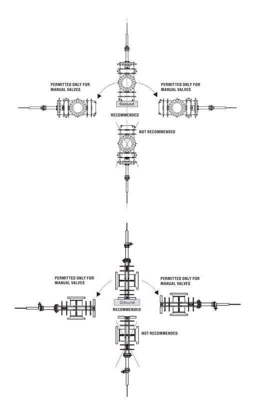
Figure 5 - Valve orientations
