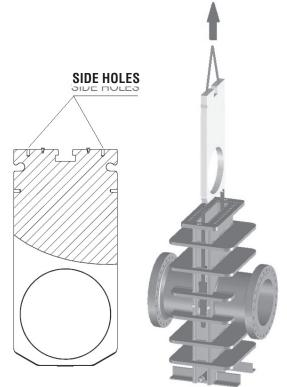
Figure 15 - Slab gate removal.
