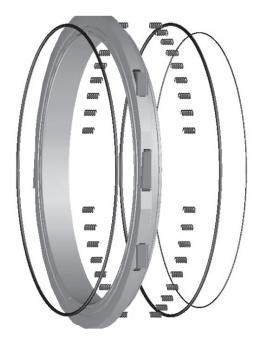
Figure 18 - Seat gaskets and springs stripping.
