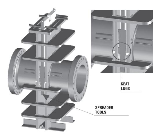
Figure 14 - Seat spreader tools use.
