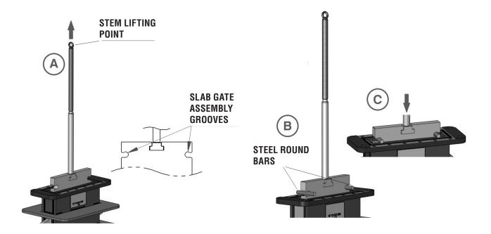
Figure 11 - Slab gate disassembly according to steps n° 12, 13 and 14.
