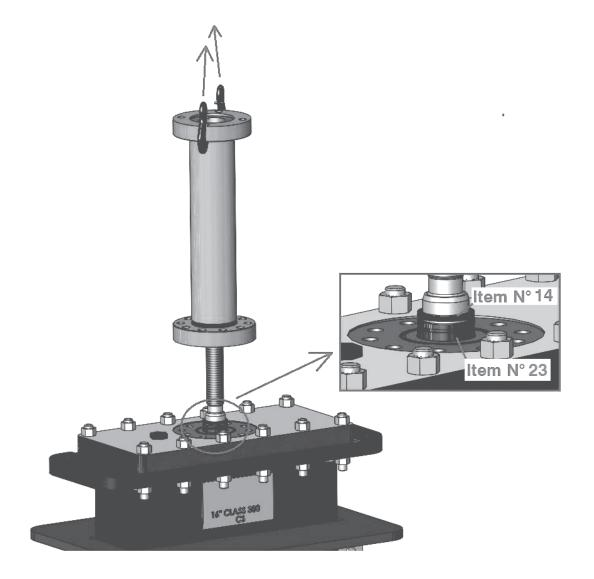
Figure 9 - Yoke disassembly and stem fire safe gasket and bearing removal.
