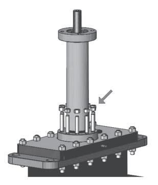
Figure 8 - Yoke bolting removal
