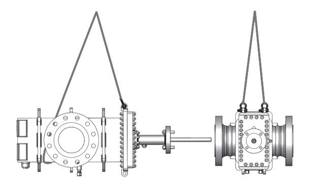
Figure 3 - Slab gate valve horizontal lifting
