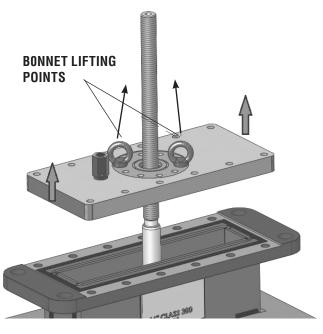
Figure 10 - Bonnet disassembly
