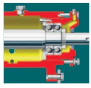
**Hook Sleeve** and replaceable metallic impeller spacer have gasket seals to isolate shaft and impeller threads from slurry. This design extends component life and eases impeller removal.
