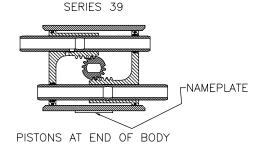
**IMPORTANT:** Note the relative location of the shaft teeth and the piston assembly's rack teeth. The above figure is viewed when looking at the top of the actuator.
