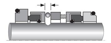
4.3 Slide the rotating seal assembly forward to **confine the ball** in the seal drive slot. See Figure 7.
