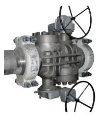
Hub Ends on High Pressure offshore applications
