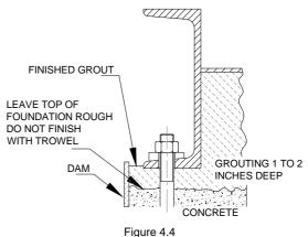
Use a good, high strength, non shrink grout mix and install as per manufacturer's instructions.
