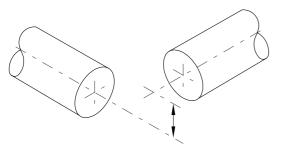
Figure 4.9 - combination of offset and angular misalignment
