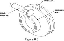
b) Make sure ring fits on impeller are free of nicks or burrs. Heat new ring to 107 °C (225 °F) and install on impeller. Drill and tap new holes in impeller spaced half the circular distance from the previously used holes in the impeller. See sketch below.
