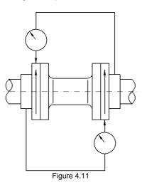
Maximum permissible misalignment at working temperature:
