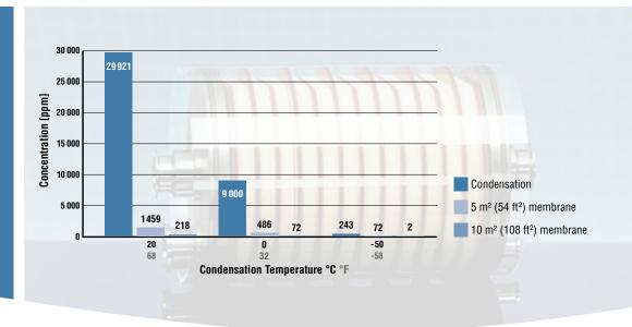
One advantage of the membrane technique versus pure condensation is the fact that the membrane process can be carried out at higher cooling-water temperatures. With a membrane, pure substances can be obtained at normal condensation temperatures that would render cryo-condensation necessary if no membrane were used. Membrane technology allows you to reduce your operating costs and recover your product!
