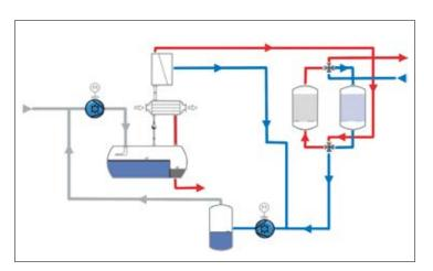
While one adsorber cleans the exhaust gas from the membrane stage, a second adsorber undergoes the regeneration process and is desorbed with the help of purging gas and negative pressure in the installed vacuum pumps. The volume of purging gas required for this is a fraction of the overall volume of gas fed into the system as a whole.
