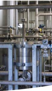
A successful combination of two processes: the hybrid plant with a membrane stage and pressure swing adsorption (PSA).
