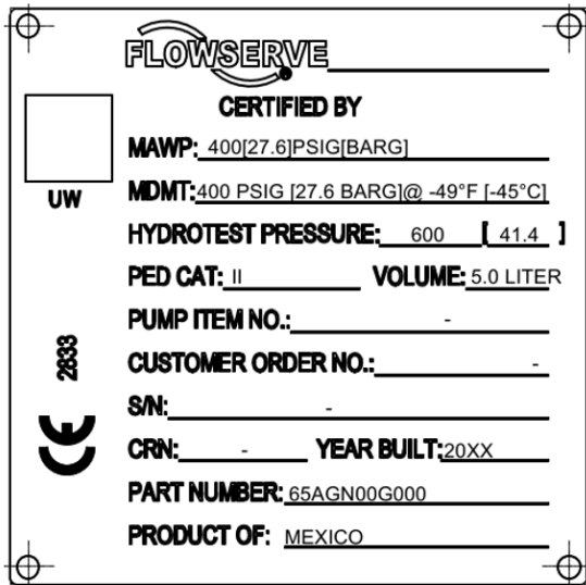
Figure 2: Example of typical nameplate
