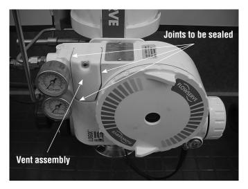
A small desiccant package as shown can be included under the sealing tape to insure proper protection.
