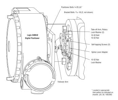
The standard rotary mounting applies to Valtek valve/actuator assemblies that do not have mounted volume tanks or handwheels. The standard mounting uses a linkage directly coupled to the valve shaft. This linkage has been designed to allow for minimal misalignment between the positioner and the actuator. The tools required for the following procedure are:
