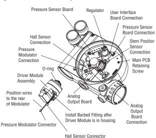
Figure 12: Driver Module Assembly
