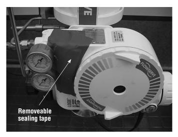
The sealing tape and desiccant should be removed when instrument air is permanently applied to the positioner.
