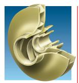
Precision Cast Closed Impeller is statically and hydraulically balanced to reduce power consumption. The impeller is keyed to shaft to provide positive drive and eliminate impeller spin-off. Balancing holes through the impeller hub minimize axial thrust and seal chamber pressure.
