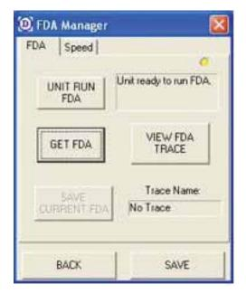
At this point, the FDA data is available for viewing. Limitorque recommends the captured data be saved for future reference for comparison analysis.
