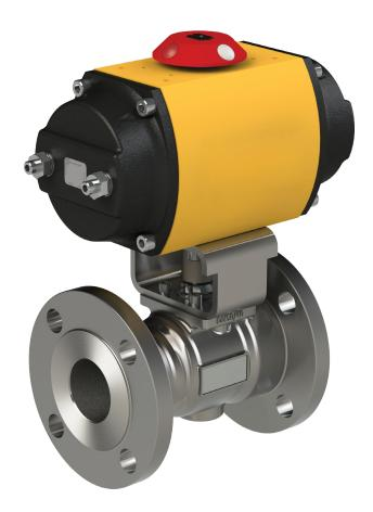
To avoid regulatory and financial risks that can occur because of fugitive emissions, Flowserve designed the Worcester 51/52 series valve to provide superior leakage resistance with a bubble-tight shutoff and a more robust, live-loaded packing design. Safety has been enhanced for end users as a result of the threaded end plug design, which ensures positive retention and eliminates any blowout risk.
