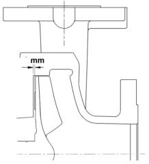
a) Before carrying out this procedure ensure that any mechanical seal(s) fitted can tolerate a change in their axial setting, otherwise it will be necessary to dismantle the unit and reset the seal axial position after adjusting the impeller back clearance.
