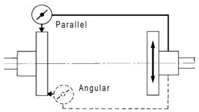
For couplings with narrow flanges use a dial indicator as shown. The alignment values are maximums for continuous service.
