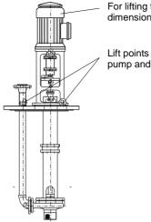
For lifting the driver refer to the dimension drawing of the driver
