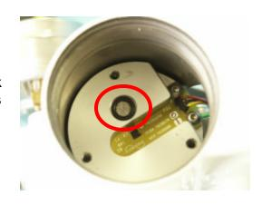
9. Replace the current standard temperature piezo assembly with the low temperature assembly (Kit Number 218956.999.000). The piezo assembly part is marked with a "-40" on the bottom of the plastic housing.
