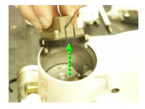
8. Verify that the O-Ring is installed in base of driver module housing (O-Ring may be stuck to the bottom of the piezo assembly that was just removed). A new O-Ring is included in the low temperature assembly kit, in the event that the original is lost or damaged during disassembly.
