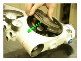
14. Perform a Quick-CAL to recalibrate the piezo assembly and the positioner. Refer to the 3200IQ IOM for detailed calibration and configuration instructions. (FCD LGAIM0058-00)
