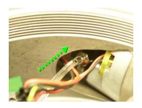
12. Insert the red and black piezo assembly connector back through the housing, and attach to the main PCB assembly, assuring the connection is tight.
