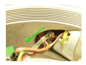
5. Pull the red and black 2-wire piezo connector through bottom of driver module housing.
