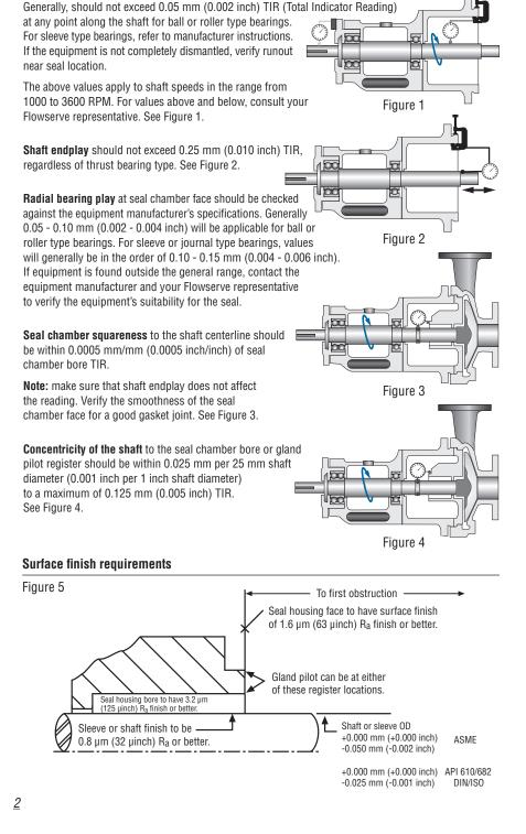
**Shaft runout** should be checked against the equipment manufacturer's specifications.
