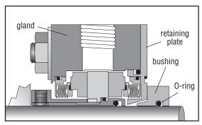
2.2 Install the pump seal chamber, Figure 8. Postion the seal gland gas barrier inlet, port A shown in Figure 9, in the 9:00 o'clock position and the plugged gas barrier outlet, port B in the 6:00 o'clock position for normal installations. Alternate positioning of the gland may be necessary with some pumps, where the bearing housing interferes with piping. Bolt the seal chamber in place on the bearing housing.
