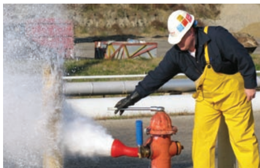
Hydraulic testing of a hydrant using a Pollard diffuser equipped with a wireless transmitter
